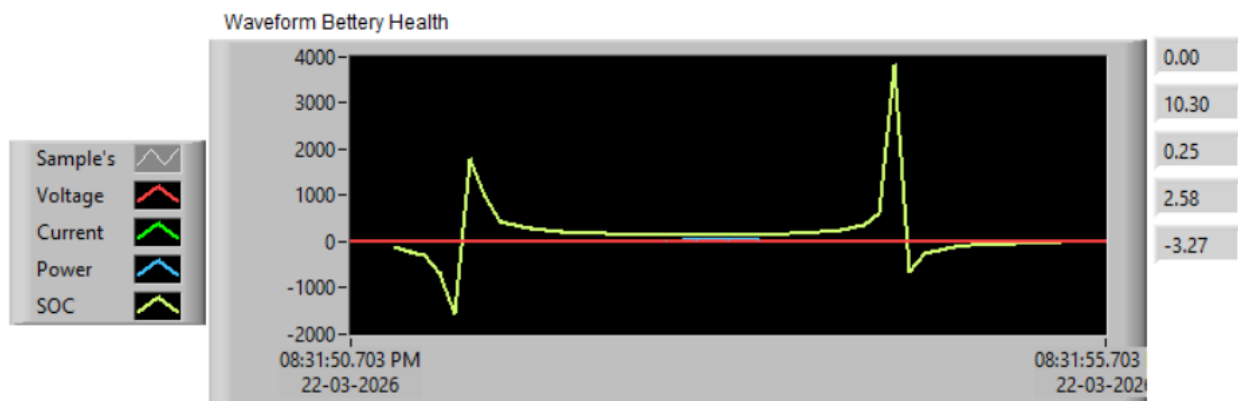
Figure 14: Real-time Waveform for Battery Health and State of Charge Monitoring
